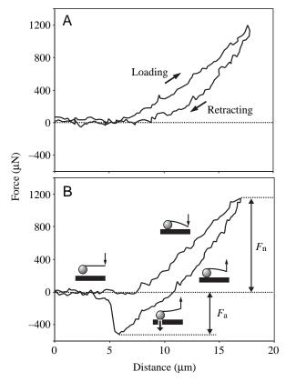
Fig. 2. Typical force–distance curves used for evaluation of elasticity and adhesive properties of the surface. (A) Without adhesion. (B) With adhesion.  $F_a$ , adhesion force;  $F_n$ , maximal applied force; Loading, part of the curve corresponding to the loading process; Retracting, part of the curve corresponding to the retracting process.
