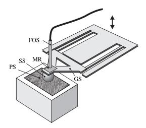
Fig. 1. Experimental set-up for estimation of material properties by microindentation. SS, sapphire sphere; FOS, fibre optical sensor; GS, glass spring; MR, mirror; PS, plant sample.
