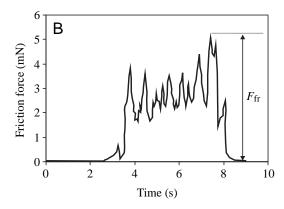
Fig. 3. Experimental set-up for friction force measurements (A) and a typical force-time curve (B) used for estimation of maximal friction force  $(F_{\rm fr})$  generated by insects. FS, force sensor; HR, hair; IN, insect; PC, computer; SC, sensor control; SP, support; TS, tested surface.
