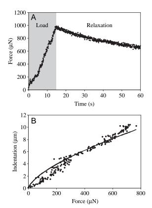
Fig. 8. Microindentation experiments on the glandular surface. (A) Force–time curve indicating that the material of the plant sample exhibited visco-elastic properties. Pitcher surface was loaded during the first 15 s (Load), then kept in contact with the upper sample for the next 45 s (Relaxation). (B) The indentation of the sample *vs* applied force (points). The solid line indicates the fit of the indentation data with the Hertz theory.
