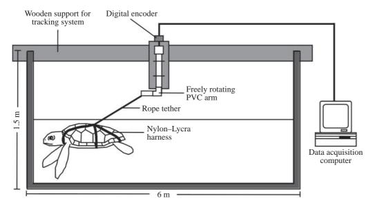
Fig. 2. Diagram experimental arena and the data acquisition system used to monitor the orientation juvenile sea turtles (turtle not drawn to scale). Each turtle was outfitted with a  $nylon-Lycra^{TM}$ harness and tethered to a rotatable arm in the arena. The data acquisition computer was located in a shed approximately 5 m to the south of the arena. See text for details.
