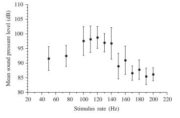
Fig. 8. Mean ( $\pm$  s.D.; *N*=2–5) sound pressure level of sounds evoked by stimulation of the sonic nerve at frequencies of 50–200 Hz. Sound pressure level was measured as the average pressure (re: 20 µPa) over the duration of a 90 ms stimulus sweep.
