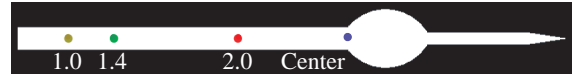
Fig. 9. Centered particles are transported more efficiently. Four simulations were run in which we measured the final position after a single cycle of a single particle placed at the mouth at time zero. The brown particle was assumed to move at mean fluid velocity as in previous simulations. The green and red particles move at 1.4 and 2.0 times mean fluid velocity, respectively, and the blue particle moves at the calculated velocity of the fluid at the center of the lumen, which varies from 2.2 to 3.5 times mean velocity depending on how open the lumen is at a particular moment. See text for further explanation.
