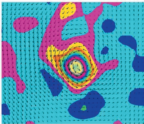
Fig. 9. Magnified view of the rightmost starting vortex in Fig. 8. The apparent centre of rotation deduced from the arrows does not lie on the peak of the spanwise vorticity.
