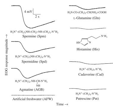
Fig. 1. Typical electro-olfactogram (EOG) responses elicited by the monoamine and polyamine odorants and the amino acid standard L-glutamine. The chemical structure, common name and abbreviation (in parentheses) of each odorant is shown below the response. The peak response was used to quantify response magnitude. All responses were obtained from the same fish. Odorants were tested at the concentration of  $100 \,\mu\text{mol} \,l^{-1}$ .
