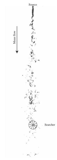
Fig. 1. Illustration of a simulated searcher in the chemical plume. The searcher's ten sensors are located at the ends of the 'spokes'. The dark patches are areas where the chemical stimulus is above threshold. The image is to scale, with the plume extending approximately 150 cm downstream of the source and the diameter of the searcher equal to 10 cm.
