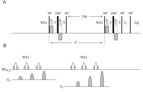
were determined by collecting a series of spectra at different amplitudes of the spatial-encoding gradients. The diffusion time was adjusted by changing the value of  $\Delta$ . Additional details are given in the text.
