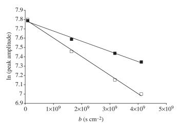
Fig. 3. Typical attenuation plot of the NMR peak amplitude as a function of the diffusion-weighting factor b in the axial (open squares) and radial (filled squares) directions in *P. argus* muscle. This example is from a measurement of arginine phosphate diffusion at a diffusion time of 150 ms. A steeper attenuation slope is indicative of a higher *D*, as seen for axial diffusion.
