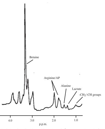
Fig. 2. A region of a lobster abdominal muscle <sup>1</sup>H-spectrum. The peaks for betaine, arginine/arginine phosphate (at 1.95 p.p.m.) and -CH<sub>2</sub>/-CH groups yielded linear attenuation plots and sufficient signal-to-noise ratios to allow measurement of D at several diffusion times. Alanine and lactate methyl peaks are also indicated for reference, although diffusion of these metabolites was not examined in the present study.
