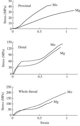
Fig. 5. Representative stress/strain curves for proximal, distal and whole threads of *Mytilus edulis* (Me) and *M. galloprovincialis* (Mg). Threads were pulled to breaking.
