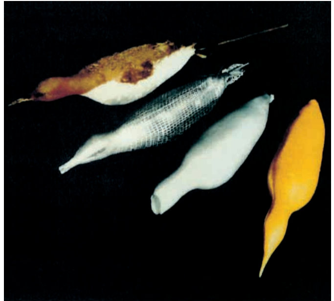
Fig. 2. Stages in the construction of the model for common guillemots, including (left to right) a frozen bird, the digitized shape averaged for five individuals, the foam carving and the finished model fitted with a cast of the bill area.
