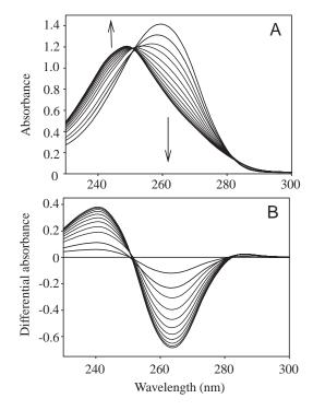
Fig. 5. Adenosine deaminase (ADA) activity in salivary homogenates of adult female *Aedes aegypti*. (A) A cuvette containing  $100 \mu mol l^{-1}$  adenosine in  $100 \mu l$  of HS buffer, pH 7.2, was scanned at 6 min intervals following addition of salivary homogenate equivalent to 0.02 of a pair of salivary glands. The arrows indicate the direction of change of the spectra over time. (B) Differential spectra for the data in A.
