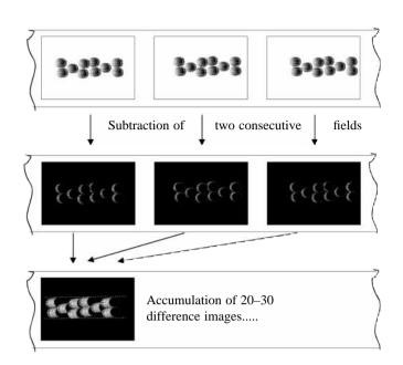
Fig. 2. Visualisation of a blood vessel by accumulation of shifting vectors from consecutive fields. The generation of difference pictures of the two fields of one frame results in the generation of shifting vectors. By superimposing a sufficiently large number of difference images from subsequent frames, a trace of all routes over which erythrocytes have travelled is obtained.
