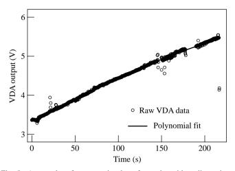
Fig. 5. A sample of raw strain data from the video dimension analyser (VDA) plotted as a function of time. A polynomial function was fitted to each set of strain data, and the function was used instead of the raw data.
