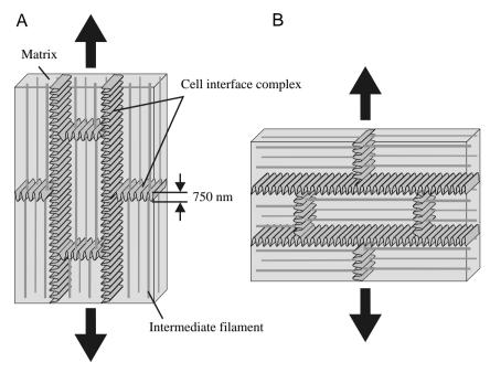
individual cells (see Fig. 11A). The agreement in stiffness between inner wall on-fibre specimens ( $E_{i,L}$ =0.42 and 0.51 GPa; Table 4) and whole tubules ( $E_{i,L}$ =0.47 GPa; Table 1) suggests that the stiffness of the complex is near the stiffness of the combined matrix and fibrous phases tested on-fibre. As a first approximation, we estimate that the stiffness of the complex is 0.5 GPa.
