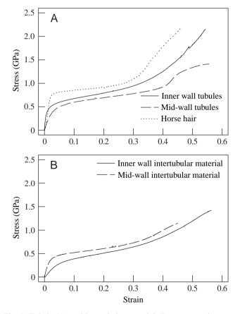
Fig. 9. Tubule (A) and intertubular material (B) stress–strain curves for inner, mid-wall and horse body hair specimens. Only representative examples are shown and they may not necessarily represent the average mechanical behaviour of the specimens.
