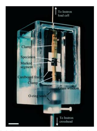
Fig. 3. The chamber used in the tensile testing of specimens of tubule dimensions. Specimens were glued to a cardboard frame using cyanoacrylate adhesive and then clamped to the test apparatus. During tests, the chamber was filled with distilled water; two O-ring oil seals mounted in the floor of the chamber permitted vertical sliding of the chamber while a specimen was mounted. Scale bar, 1 cm.
