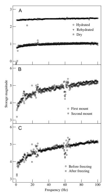
Fig. 8. Storage magnitude (analogous to E') plotted against test frequency. The effects of dehydration (A) and of freezing (C) were negligible; artefacts resulting from mounting inconsistencies (B) were sufficient to explain slight differences before and after treatment. The artefacts at approximately 30 Hz and 60 Hz are the result of 60 Hz electrical noise in the system.
