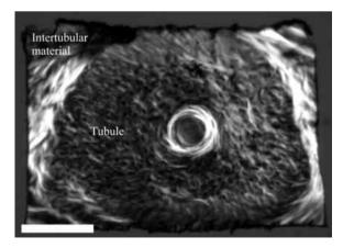
Fig. 4. A video-captured cross-sectional image of a tubule test specimen from the inner hoof wall. Inclusion of intertubular material with tubule specimens was unavoidable; the reverse was also occasionally the case. Scale bar,  $100 \,\mu$ m.
