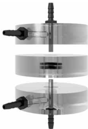
Fig. 1. Model-membrane apparatus, shown partially unassembled. All three sections are solid acrylic disks with hollowed-out core sections. The upper and lower disks are drilled to accept gas-tight copper tubing connectors. Air entered and exited the apparatus only through the top two ports, and water circulated only through the lower two ports. The membrane was held in the center section by silicone gaskets, which were in turn held in place by a large plastic retaining ring. The upper surface of the membrane was therefore exposed to dry air blown through the ports in the upper section, and the lower surface of the membrane was in contact with the water circulating within the lower section of the apparatus.
