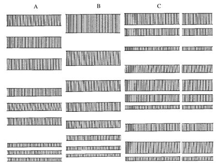
Fig. 1. Three ways of achieving a broadband, wavelength-independent reflectance in a multilayer stack. High refractive index material is shown shaded. (A) Three regular multilayer stacks, each tuned to a different wavelength. (B) A 'chirped' stack. (C) A 'chaotic' stack. See text for explanations of each reflector.
