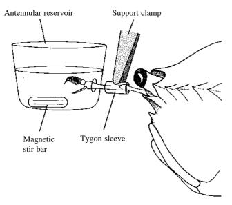
Fig. 2. Schematic diagram of the apparatus used to examine tracer flux between the hemolymph and the sensillar lymph, and to measure trans-antennule potential. The crab (shown to the right) was secured to a stable platform and remained out of water during the course of an experiment.
