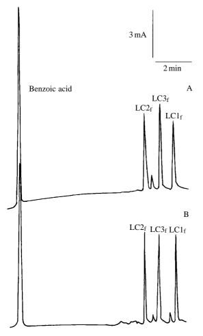
Fig. 8. Separation of myosin light chains from the fast muscle of a 15 °C-acclimated short-horned sculpin by SDS–capillary electrophoresis using an internal benzoic acid standard (see text for details). (A) Purified myosin from 5 °C-acclimated fish; (B) purified myosin from 15 °C-acclimated fish. LC1<sub>f</sub> and LC3<sub>f</sub>, alkali light chains of myosin; LC2<sub>f</sub>, regulatory myosin light chain.
