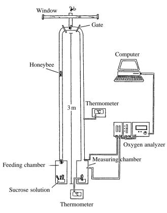
Fig. 2. Diagram of the experimental arrangement. The tube system is seen from above. After entering the tube outside the laboratory window, individuals can be gated either to the feeding or to the measuring chamber (after Esch *et al.* 1994).
