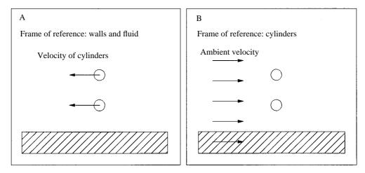
Fig. 3. The flow field relative to a pair of cylinders (observed from the cylinders' frame of reference) will be the same whether the cylinders are moving with respect to stationary surroundings (A) or the surroundings are moving with respect to stationary cylinders (B).
