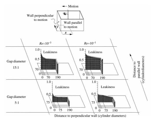
Fig. 10. Leakiness (z axis, vertical) as a function of position in experimental tank; the distances to all four walls are indicated by the position relative to the four sides of the x,y rectangle.
