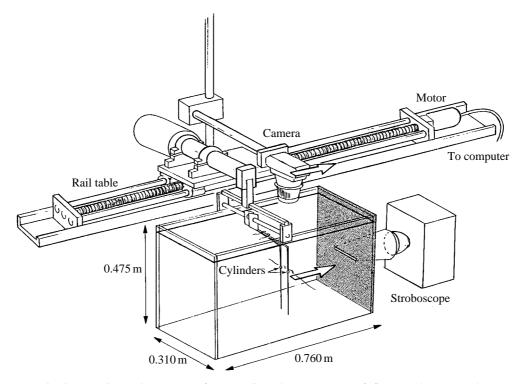
Fig. 2. Experimental apparatus for recording the movement of flow markers past the cylinders. The camera was stationed above, and moved with, the cylinders (movement indicated by arrows). This movement was driven by a motorized rail table controlled by a computer. Flashing light from a stroboscope entered the tank through a horizontal slit.
