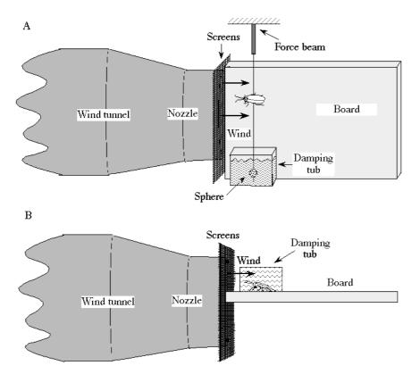
Fig. 1. Diagram of cockroach in working section of wind tunnel, as described in the text. (A) Side view of the wind tunnel. (B) Top view of the wind tunnel.
