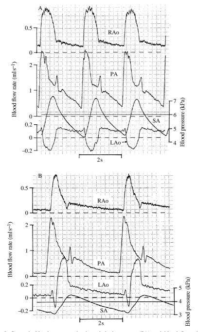
Fig. 8. Systemic blood pressures in the subclavian artery (SA) and blood flows in the pulmonary artery (PA), right aorta (RAo) and left aorta (LAo) to show the differences between (A) an unanaesthetized alert animal (2.4kg), in full view in the laboratory, and (B) the same animal, calm and resting behind a screen. A R-to-L shunt is established in B and is associated with bradycardia and systemic hypotension.
