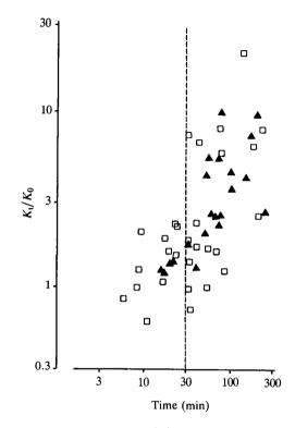
Fig. 6. The increase in relaxation rate (K) during phase 2 with time. The vertical axis represents the current rate  $(K_1)$  as a multiple of initial rate  $(K_0)$ . The steady increase in compliance with time could be minimised by limiting distensions to brief periods using a distension pressure 0.4-0.6 kPa. Squares, *in vitro*; triangles, *in situ*. Note that the axes are logarithmic. Vertical dashed line represents the point at which relaxation rate starts to rise.
