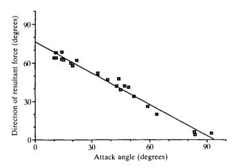
Fig. 3. Direction of the aerodynamic force acting on a moderately large specimen of *Velella velella* as a function of the attack angle of the sail; (y=-0.8x+76.7; r=0.99). Force direction is measured as a counterclockwise angle in relation to wind direction.
