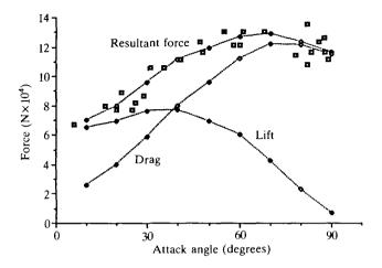
Fig. 2. Total (horizontal) aerodynamic force acting on a moderately large specimen of *Velella velella* (maximum sail length, 57 mm) at near-surface windspeeds of  $1.3 \text{ m s}^{-1}$ , measured as a function of the animal's orientation (attack angle of the sail). A line was fitted by connecting average points (small squares) calculated after rounding attack angles to the nearest 10°. Lift and drag components were calculated from direct measurements of force magnitude and direction.
