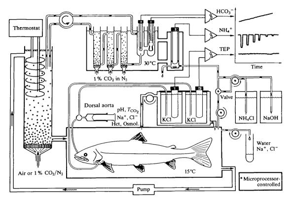
Fig. 1. Experimental apparatus showing the recirculating water system and apparatus used for automated determination of  $[HCO_3^-]$  and  $[NH_4^+]$  in the water. See text for details. TEP, transepithelial potential;  $T_{CO_2}$ , total CO<sub>2</sub> concentration; Osmol, osmolarity.
