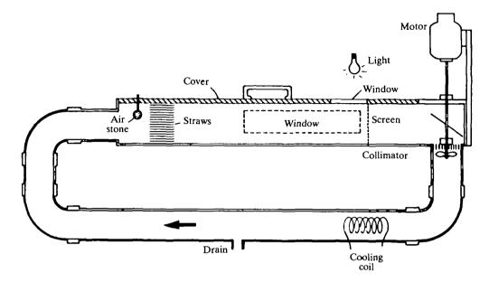
Fig. 1. Schematic diagram of the swim chamber designed after Vogel & LaBarbera (1978). Arrow shows direction of water flow.
