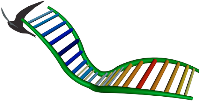
Fig. 10. Three-dimensional wake structure of the swift in cruising flight. The image frame is as if the bird flew obliquely from right to left and slightly into the paper, leaving the trace of one wingbeat in still air, starting at the upper turning point. Green tubes show the wingtip vortices, cylinders in shades of red are spanwise vortices with positive circulation and cylinders in shades of blue have negative circulation. The colour intensities and tube diameters are proportional to the strengths of each component. The geometry is deduced from a combination of wingbeat kinematics and streamwise plane section data.
