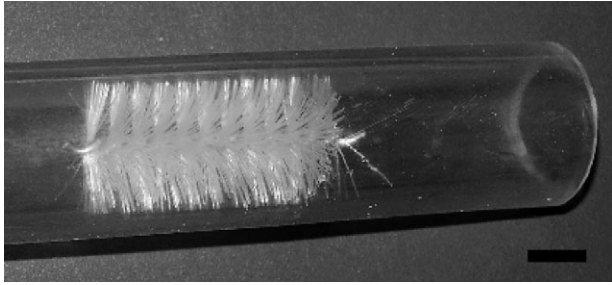
Fig. 1. Apparatus for measuring the effects of hagfish slime on flow rate through and resistance across an artificial gill analogue, which consisted of a piece of test tube brush within polyvinyl tubing. Scale bar, 10 mm.
