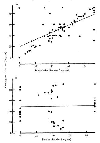
Fig. 7. (A) Linear regression analysis of intertubular material orientation versus crack growth direction (both relative to precut notch). r = 0.68; N = 119; t = 10.02; P < 0.05. (B) Linear regression analysis of tubular orientation versus crack growth direction (both relative to precut notch). Slope not significant.
