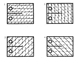
Fig. 4. Diagram of the relationship between the precut notch of the CT specimen and tubular and intertubular material for the four sample orientations used. Note that orientations 1 and 2 or 3 and 4 could be cut from the same sample by altering the direction of the notch. Tubular material orientation is designated by solid lines, intertubular orientation by dashed lines.
