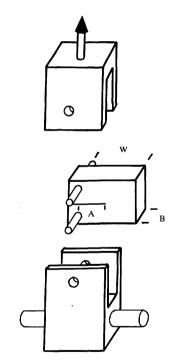
Fig. 3. Compact tension fracture test (CT) specimen and exploded view of loading clevis. B, full width of specimen; W, full ligament length measured from centre of loading pins to edge of specimen; A, notch length measured from centre of loading pins to end of precut notch. Lower clevis is secured to test chamber and test machine moving crosshead. Upper clevis is attached to 500 kg maximum force transducer.
