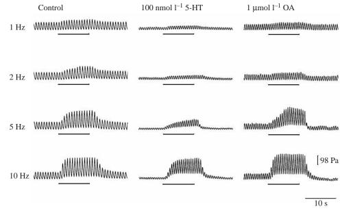
Fig. 6. Effects of stimulation of the fifth lateral cardiac nerve (LCN5) on pressure pulses recorded from the fifth lateral artery (LA5) during perfusion of SW (control), serotonin (5-HT) and octopamine (OA). These data were obtained from one preparation. Bars show the periods of stimulation. Frequencies of stimulation are shown at the beginning of the traces in the left column.
