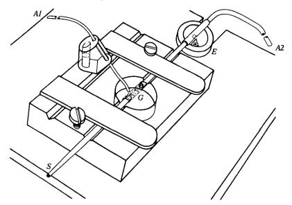
Fig. 1. Apparatus for flux measurements. G, isolated midgut. A1, A2; Ringer agar-agar bridges going to calomel cells and voltmeter; S, connection to a precision syringe by plastic tubing; E, Eppendorf vial to collect lumen solution dropping down.
