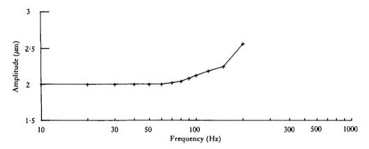
Fig. 1. Frequency response of the stimulus probe to a 10 V driving voltage.
