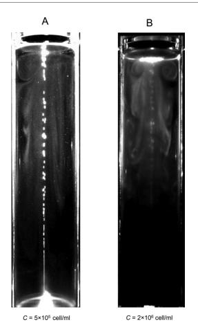
Fig. 4. Increased cell suspension density leads to a smaller vortical ring distribution. Instantaneous images showing that in a lower density of cells (C=5×10<sup>5</sup> cells/ml), vortical distribution near the free surface extends to the cylinder wall. However, in a higher density of cells (C=2×10<sup>6</sup> cells/ml), the vortical distribution did not reach the wall, indicating a smaller vortical ring (bubble flow rate Q=100 µl/min, diameter D=40 mm, with blue light).
