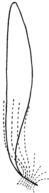
Fig. 3. Diagrammatic representation of the flow of water induced by the caudal fin of a dolphin or fish.
