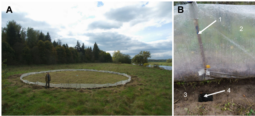
Fig. 2. Circular arena for the experiments. Overall view (A) and construction (B). 1, wooden stake; 2, polyethylene wall; 3, groove; 4, trap.
