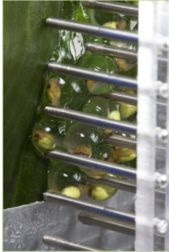
Fig. S3. Agalychnis callidryas egg clutch set up for vibration playback. Clutches were mounted vertically, then a set of blunt metal tines connected to a shaker were inserted among the eggs to deliver the vibrational stimulus.
