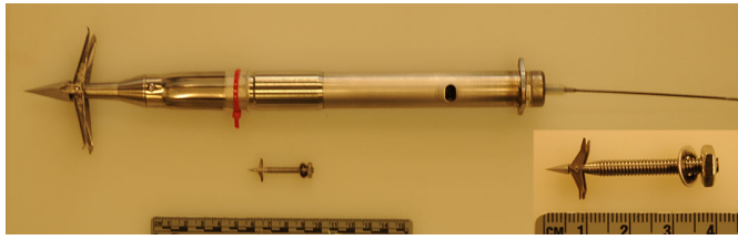
Fig. 4. Large whale tracking tag and 1/7th scaled dolphin dummy tag. Inset shows dummy tag at a larger scale. Scales in cm.
