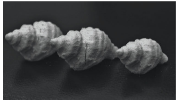
Fig. 6. Evident fracture patterns in Nucella shell models. Printed and live gastropods consistently showed crack formation at the base of the spire in almost all trials. Crack propagation continued dorsally along the spire suture, paralleling the shell aperture. This pattern was repeated across shells regardless of shell size.
